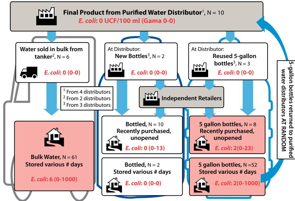
Figure 6. Diagram of water distribution system in Puerto Ayora.
