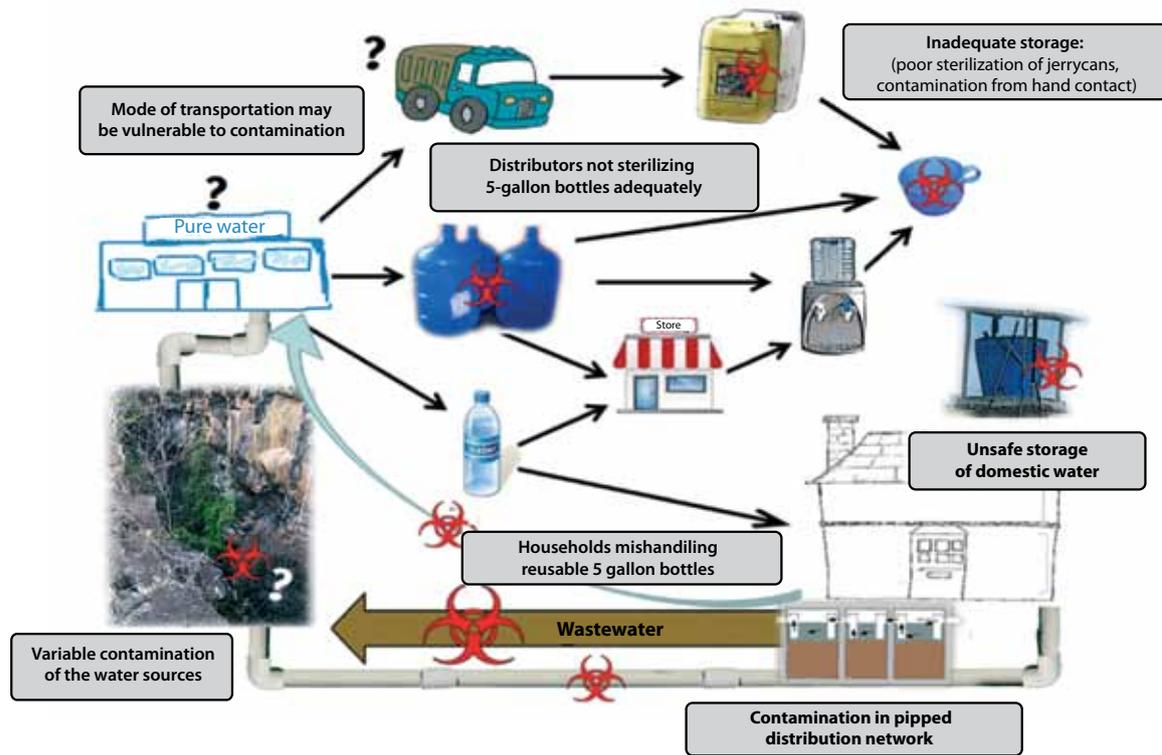
**Figure 9.** Diagram of the current water flow model for domestic and potable water from source to sink in Puerto Ayora and weak points in the system.
