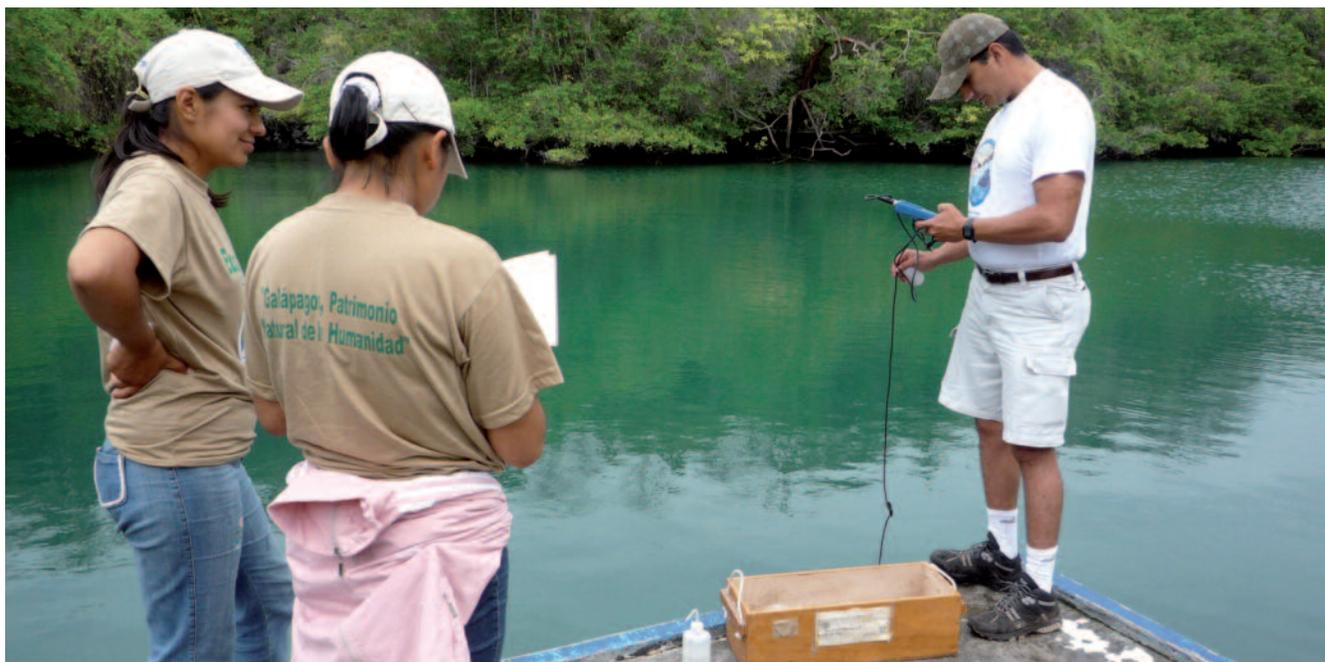
**Figure 1.** Measuring dissolved oxygen and pH of the water in the Ninfas Lagoon, Santa Cruz.
